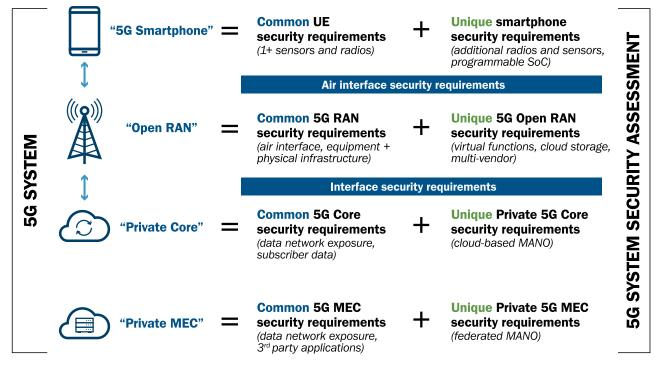
Figure 2. Top-Level 5G System Reference Design
